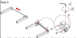
Insert the other side of the Hexagonal rod into the hexagonal hole of the Left lifting leg (part 3), and attach the Crossbeam (part 6) to the Lifting leg (part 2 and 3) using (part A) Screw M6x10.
