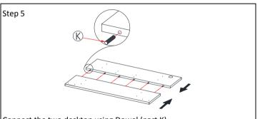
Connect the two desktop using Dowel (part K).
