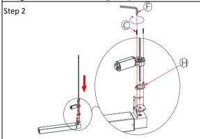
Insert the Hexagonal rod assembled in Step 1 into the hexagonal hole of the Right lifting leg (part 2) through the Motor Gasket (part H), and tighten it with (part C) Screw M5x30.
