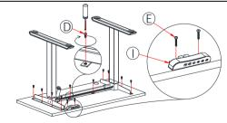
Adjust Crossbeams to proper position to fit the desktop. Tighten the (part D) Wood screw ST4.8x16 to lock. Attach the Handset (part I) to the underside of the desktop using (part E) Wood screw ST4.2x16.
