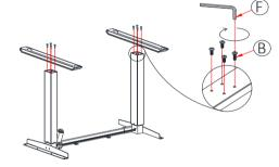
Attach Foot (part 1) to the Lifting leg (part 2 and 3) using (part B) Screw M6x16.
