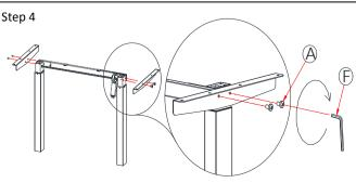
Attach Side bracket (part 4) to the Crossbeam (part 6) using (part A) Screw M6x10.
